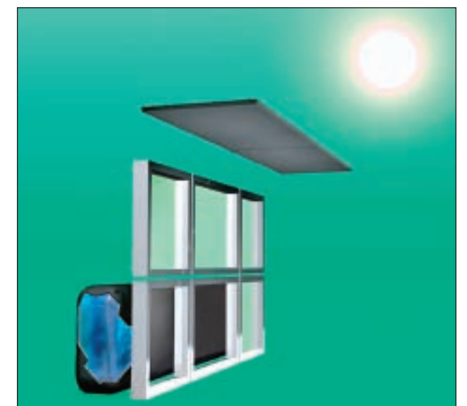
[Above] Cal Poly used a black water tank, (a type of Trombe Wall) as thermal mass. In winter, the lower sun shines directly on the tank, and heats the water. At night the warm water radiates heat into the house.
