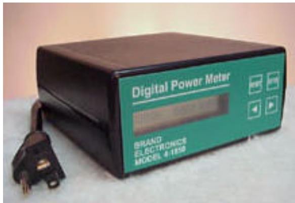
Fig. 4. kWh Plug Load Meters - Top) P3 Killawatt Plug Meter; (Middle) spreadsheet graph generated from data collected by data logger; (Below) - Brand Power Meter – data logger w/PC interface
