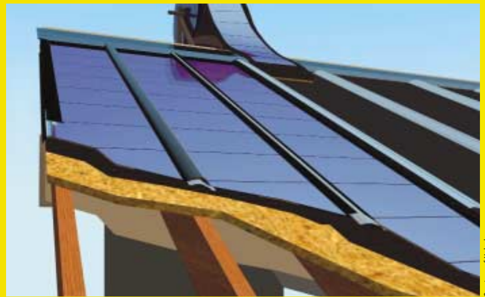
The flexible panels become the primary roofing material, as shown in this rendering.
